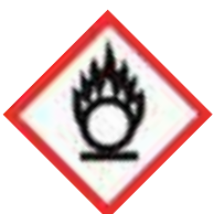
Flame over set e.g. Oxidizing solids
